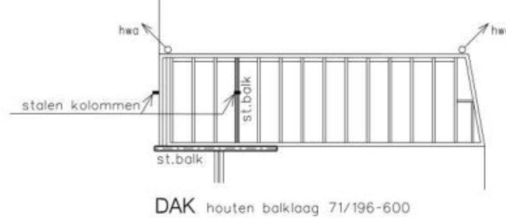
DAK houten balklaag 71/196-600
